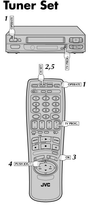
Your recorder needs to memorise all necessary stations in preset positions in order to record TV programmes. ATS+ (Auto Tuning System) automatically assigns all receivable stations in your area to call them up with the TV PROG. buttons without going through any vacant channels.
